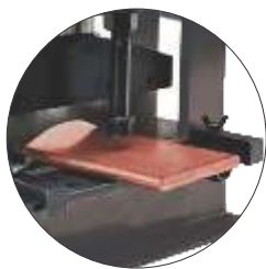
Bus Bar Cutting
