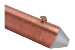
Adhesion Test: An 18-inch length of the rod with one end cut to a 45 degree point shall be driven between two steel clamping plates or the jaws of a vise, set 0.04 inch less than the diameter of the rod, so as to shear off sufficient metal to expose the bond between the jacket and rod. Peeling of the jacket by the steel plates or the jaws of the vise is acceptable, but there shall be no other evidence of separation of the jacket from the steel core.
